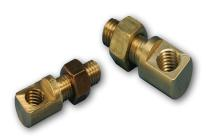
Extendable adapter provides an additional 2" offset when used with air terminal bases. Can be coupled with LPx291 -LPx295 series to provide a total of 3" offset.
