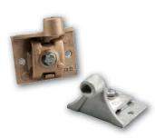
Bronze or aluminum cast point base for use on vertical surface with horizontal or vertical run of cable. Point attachment offset 2" from surface to clear overhang of wall cap or cover. Positive bolt tension cable clamping with two.281" diameter mounting holes for bolts or screws.
