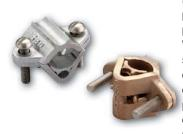
Bronze or aluminum cast pipe mount point for vertical pipe or cable pipe bond. When used as a point support it may be used with or without cable run on pipe or will allow point to stand off pipe to use type 321 point to cable connector. Maximum mounting diameter of 1.75".
