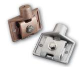
Bronze or aluminum cast point base for use on vertical surface with horizontal or vertical run of cable. Positive bolt tension cable clamping with two.281" diameter mounting holes for bolts or screws.
