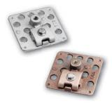
Bronze or aluminum cast adhesive point base for use on flat surfaces when no penetration may be made for anchoring. Positive single bolt tension cable clamping. For use with hot pitch, roofing compound or commercial adhesive on built-up roof surfaces or other locations.
