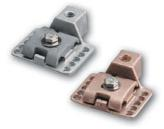
Bronze or aluminum cast adhesive point base for use on flat or vertical surfaces. Positive single bolt tension for multidirectional cable clamping. Four.250" diameter mounting holes for bolts or screws.
