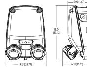
EXTL SP640L/ SP1100L/SP2200L Specifications Length: 10.42(26.47) Depth: 6.42(15.85) Height: 13.94(35.41) Weight of SP640L / SP1100L: 5.55lbs (2.52kg) Weight of LP2200L: 7.65 lbs (3.47kg)
