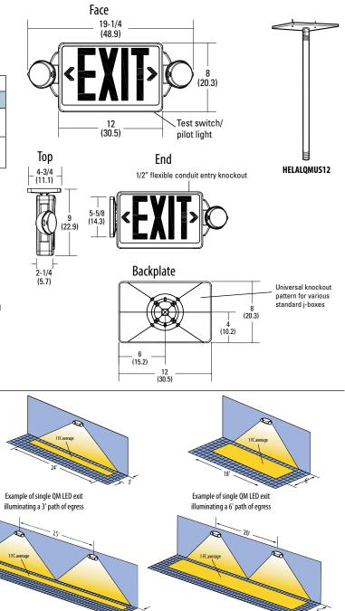
MULTIPLE COVERAGE 3W Total White LEDs Using multiple units at a typical 7.5' mounting height delivers 25' center-to-center spacing on a 3' path of egress and 20' center-to-center spacing on a 6' path of egress.
